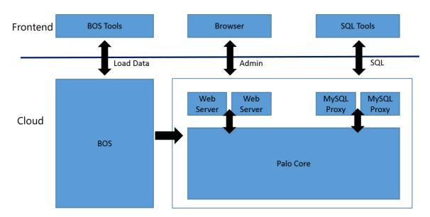
External products of Palo, Baidu Data Warehouse, consist of cloud and frontend. The frontend provides users with tools to interact with the cloud, which can upload data to BOS, perform Palo cluster management and submit SQL statements.
