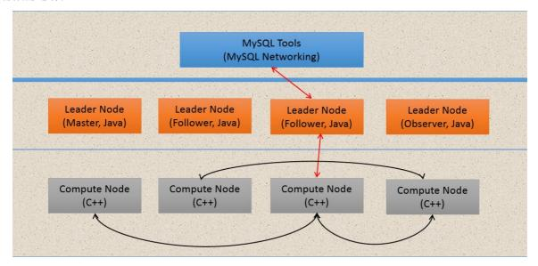
Palo Core is mainly divided into two roles, i.e., Leader Node and Compute Node, each of which can be deployed on multiple machines.
